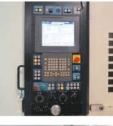
2007 MAKINO A71 4-Axis, Fanuc Pro 5 Control, Travels: X28.7", Y-28.7", Z 31.5", (2) 19.7" Pallets, 10,000 RPM, 25 HP, Cat 50, 60 ATC, Rapid Traverse & Feed Rates 1,969 IPM, Max Workpiece 31.5"x 39.4", Coolant Through Spindle, sn 481
