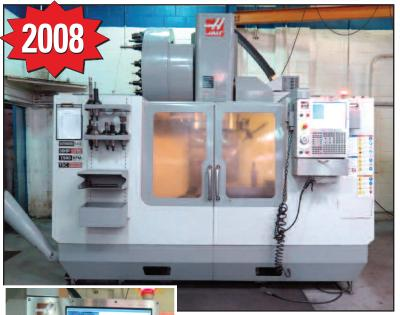
• 2008 HAAS VF-3YT-50 4-Axis, Travels: X-40", Y-26", Z-25", Table Size 52"x23", 7,500 RPM, Cat 50, 30 ATC Side Mount, Spindle Nose To Table 7.9"-32.9", Table Cap. 4,000 lbs, Rapid Feed Rate 710 IPM, Max Cutting Rate 500 IPM, Coolant Through Spindle, Chip Auger, Coolant, 30 HP, sn 1068144
