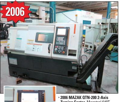
• 2006 MAZAK QTN-200 2-Axis Turning Center, Mazatrol 640T Nexus Control, 24" Swing, 20.2" Max Turning Length, 13.8" Max Turning Diam., Travels: X-8.7", Z-21.1", 8" Chuck, 2.9" Bore, 12 Station Turret, 4,200 RPM, Tailstock, Tool Setter, Chip Conveyor, 35 HP, sn 182582
