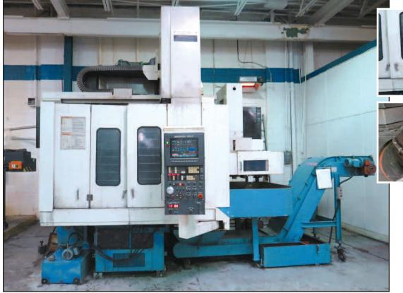
MAZAK Megaturn A-12 CNC Vertical Turning Center, Mazatrol T32-2 Control, 49.2" Chuck, 57.1" Max Swing, 48.2" Max Height Under Rail, 48" Max Cutting Height, 350 RPM, 16 ATC, Coolant Through Spindle, 30 HP, sn 90796
