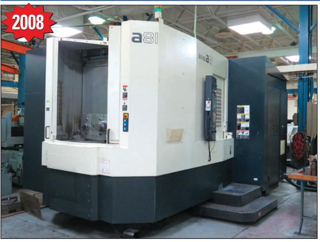
• 2008 MAKINO A81 4-Axis, Fanuc Pro 5 Control, Travels: X-35.4", Y-31.5", Z-35.4", (2) 24.8" Pallets, 10,000 RPM, Cat 50, 60 ATC, Rapid Traverse & Feed Rates 1,969 IPM, Max Workpiece 39.4"x 51.2", High Pressure Coolant Through Spindle, Chip Conveyor, sn 630
