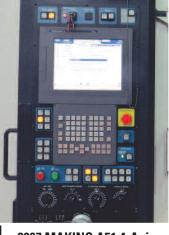
• 2007 MAKINO A51 4-Axis, Fanuc Pro 5 Control, Travels: X-22", Y-22", Z-19.7", (2) 15.7" Pallets, 14,000 RPM, 30 HP, Cat 40, 60 ATC, Rapid Traverse 2,362 IPM, Feed Rate 1,968 IPM, Max Workpiece 24.8"x 35.4", Coolant Through Spindle, sn 793
