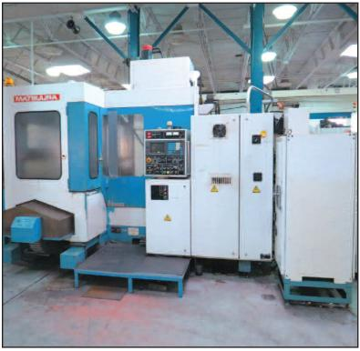
• MATSUURA MC900H-63-PC2S 4-Axis, Fanuc 15M Control, Travels: X-36.2", Y-28.3", Z-30", (2) 24.8" Pallets, Pallet Indexing 0.001 Degree, Max Pallet Load 2,645 lbs, 4,500 RPM, Cat 50, 50 ATC, Table Top To Spindle Center 2.9"-31.3", Coolant Through Spindle, Chip Conveyor, 20 HP, sn 890407985
