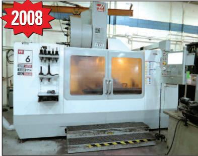
• 2008 HAAS VF-6/50 4-Axis, Travels: X-64", Y-32", Z-30", Table Size 64"x28", 7,500 RPM, Cat 50, 30 ATC Side Mount, Spindle Nose To Table 5"-35", Table Cap. 4,000 lbs, Rapid Feed Rate 600 IPM, Max Cutting Rate 500 IPM, Coolant Through Spindle, Chip Auger, 30 HP, sn 1067789
