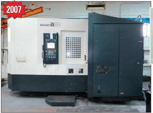
• 2007 MAKINO A81 4-Axis, Fanuc Pro 5 Control, Travels: X-35.4", Y-31.5", Z-40.2", (2) 24.8" Pallets, 10,000 RPM, Cat 50, 60 ATC, Rapid Traverse & Feed Rates 1,969 IPM, Max Workpiece 39.4"x 51.2", High Pressure Coolant Through Spindle, Chip Conveyor, sn 213
