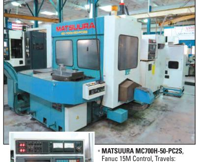
MATSUURA MC700H-50-PC2S, Fanuc 15M Control, Travels: X-29.5", Y-24", Z-25", (2) 19.7" Pallets, 4-Axis, 4,500 RPM, 15 HP, Coolant Through Spindle, Cat 50, 50 ATC, Chip Conveyor, sn 890407902
