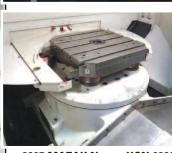
• 2005 MAZAK Nexus HCN 6000 4-Axis, Mazatrol Fusion 640M Nexus Control, Travels: X-31.5", Y-31.5", Z-31.5", (2) 19.7" Pallets, 10,000 RPM Hi-Torque Spindle, Cat 50, 60 ATC, Max Workpiece 35.4"x 39.4", High Pressure Coolant Through Spindle, Chip Conveyor, 50 HP, sn 179848
