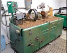
MAGNAFLUX AN 04845AO Magnetic Particle Inspection
