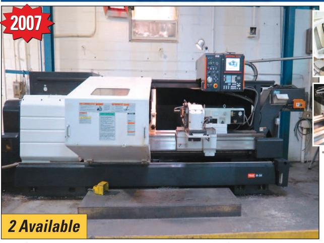
• (2) 2007 MAZAK M-5N-2000 Flat Bed CNC Lathes, Mazatrol 640T Control, Travels: X-22.1", Z-80.9", W-5.1", 4.1" Spindle Bore, 24" Swing, 81.9" Max Turning Length, 24" Chuck, 2,200 RPM, Horiz. & Vert. Turrets, 8 Station Turret, 6 Station Chucker, Tool Eye, Steady Rest, Chip Conveyor, 30 HP, sn's 198318 & 195906
