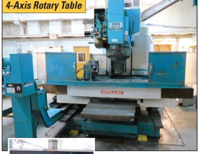
MATSUURA MC-1500V4, Fanuc 11M Control, Travels: X-60.2", Y-30.7", Z-29.5", Table Size 66.9"x 29.9", 3,500 RPM, BT-45 Taper, 40 ATC, Spindle Nose to Table 7.8"-37.4", Table Capacity 5,500 lbs, Rapid Traverse (X/Y) 472 IPM, Feed Rate 157 IPM, Chip Conveyor, 4th Axis Attachment, 25 HP, sn 890307897
